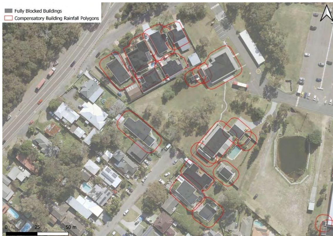
Figure 4 An Example of Removed Buildings and the Compensatory Building Rainfall Polygons
