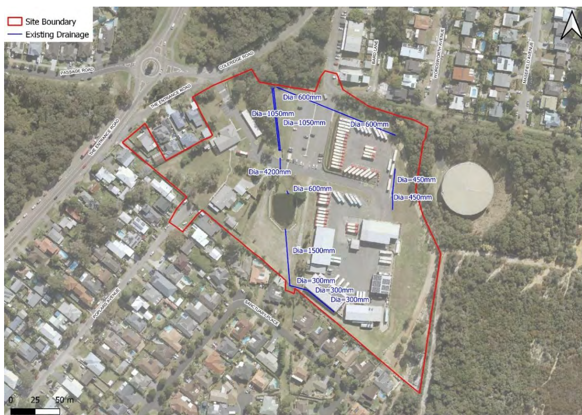
Figure 5 Layout of the Existing Drainage Network included in the TUFLOW Floodplain Model
